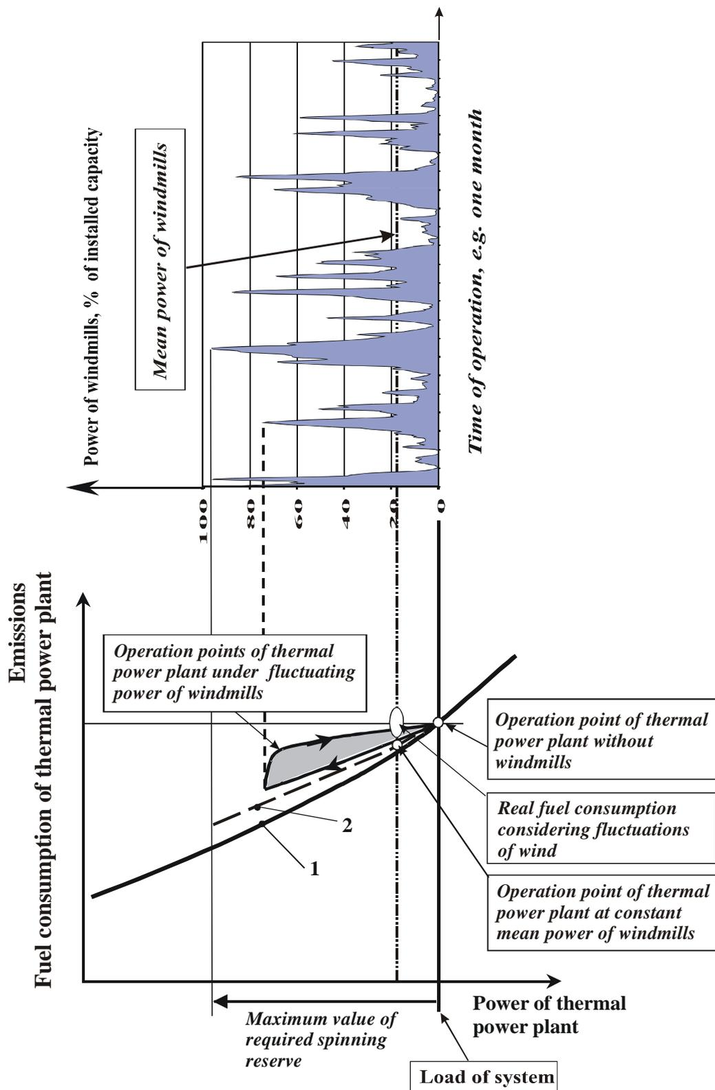
Fig.3. Explanation of wind energy balancing and fuel consumption increase problem.
