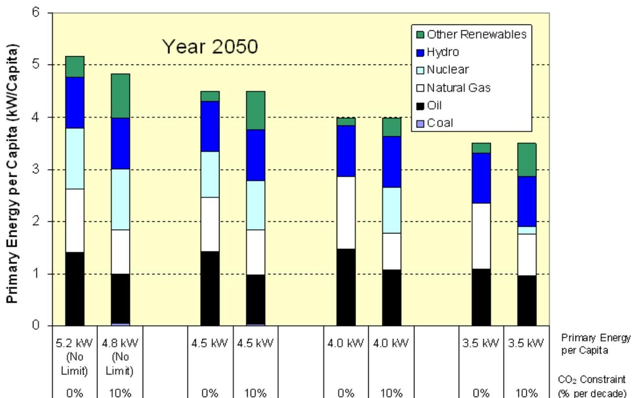
Figure 4: Primary energy per capita mix in Switzerland in the year 2050 for scenarios with an increasingly stringent constraint on primary energy per capita (labelled “no limit” to “3.5 kW”) imposed in isolation and in combination with a reduction on CO<sub>2</sub> emissions of 10% per decade up to the year 2050.
