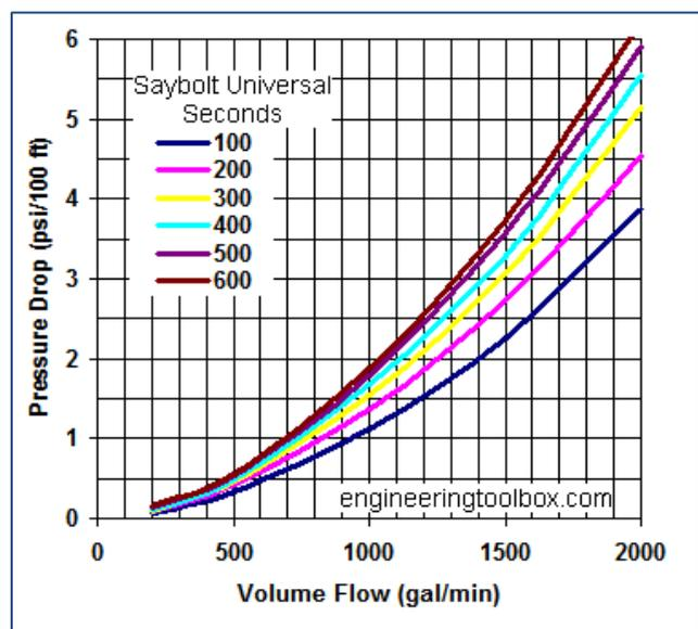
Figure 1 – Pressure drop in 6"-inner-dia oil pipelines [12]
