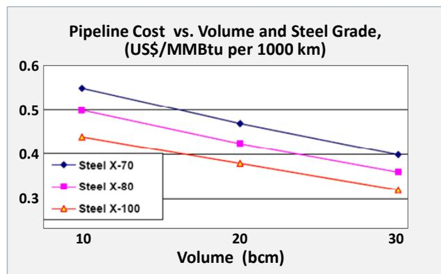
Fig. 4 – Pipeline transportation cost for a 1000 km pipeline as a function of volume and steel grade [29]
