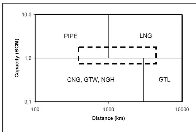
Figure 2 – Capacity-Distance Diagram for Natural Gas Transportation Technologies [17]
