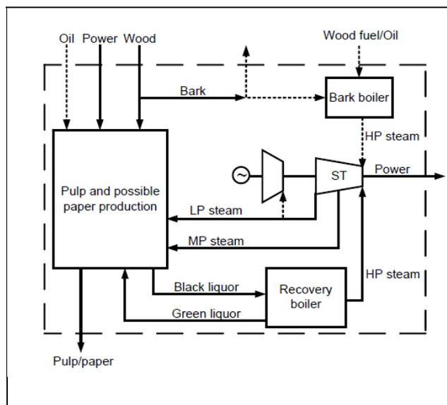
**Figure 1.** Main energy and material streams at a conventional kraft pulp mill with a recovery boiler. (Pettersson, 2011) [2]
