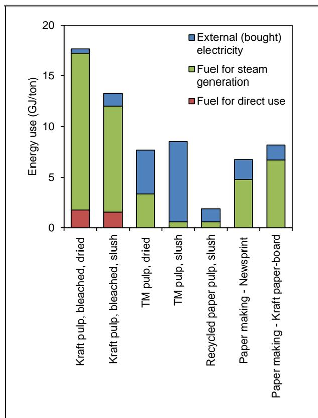
Figure 5. Specific energy use for different pulp and paper production processes. Values are averages for mills in Sweden in 2007. (Wiberg, 2012) [4]
