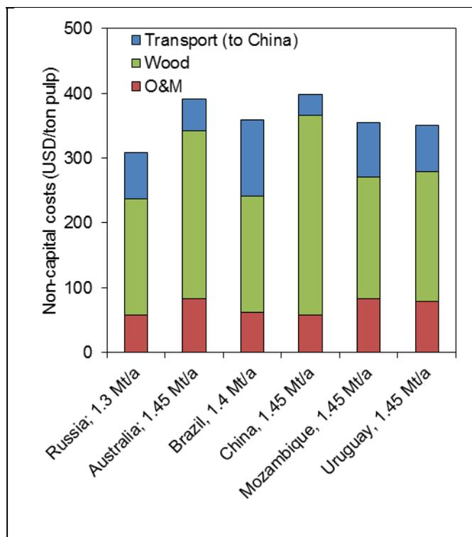
Figure 8. Operation and maintenance costs (O&M), pulpwood costs, and pulp transport cost for large scale (1.3-1.5 Mt/a) greenfield pulpmills for different locations and capacities. (EBRD & PÖYRY, 2012) [10]
