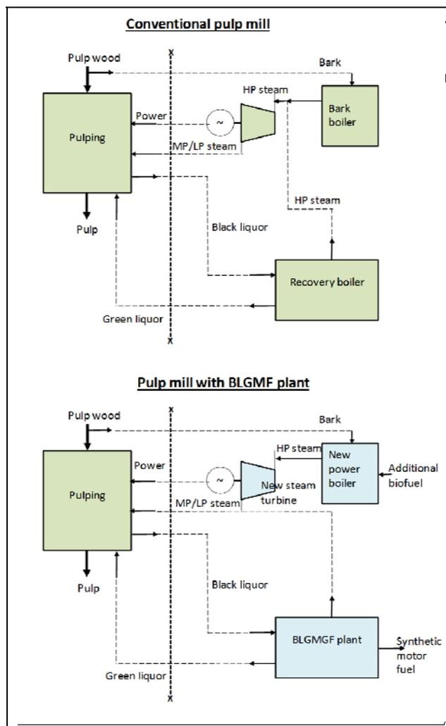
Figure 6. An overview of the principal differences between a conventional pulp mill and a mill with BLGMF plant according to Ekbohm et al. (2005) [9].
