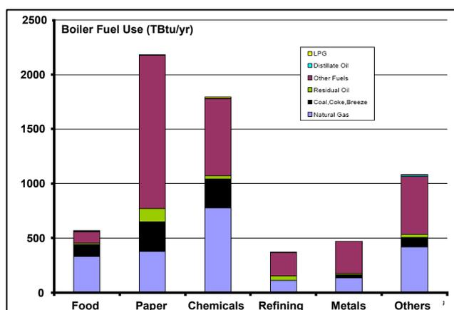
Fig. 3 – Boiler fuel use in the US industry by sector [2]
