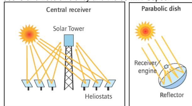
Figure 3 – Solar Tower and Solar Dish Concepts
