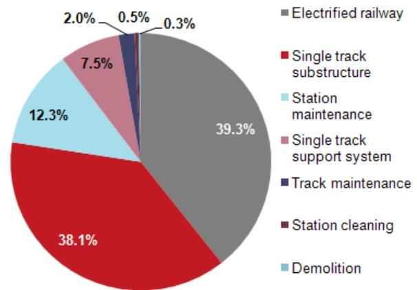
**Figure 2 Split of maintenance energy consumption per track km for electrified rail [17, 18].**
