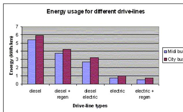
Figure 2 – UK bus energy usage for different powertrains [24]
