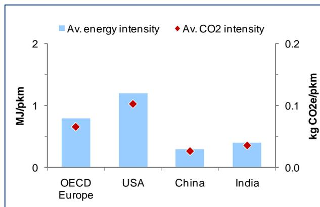
Figure 1 – Energy and CO<sub>2</sub> intensity of buses [1]
