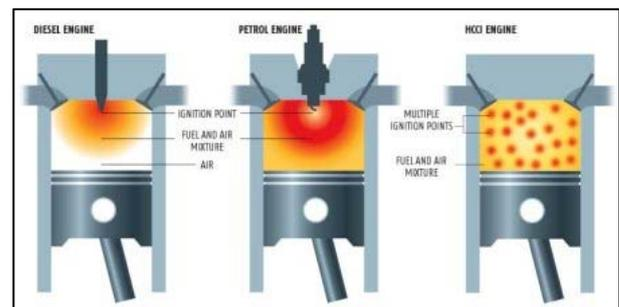
Fig. 1 - Diesel, Petrol and HCCI Engine
