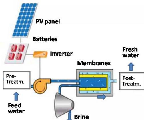
Figure 6 - Coupled PV and RO desalination plants (Al-Karaghoul et al., 2011)
