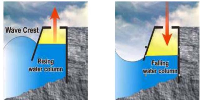
Fig 2 - Oscillating water column concept (Mueller et al, 2007)
