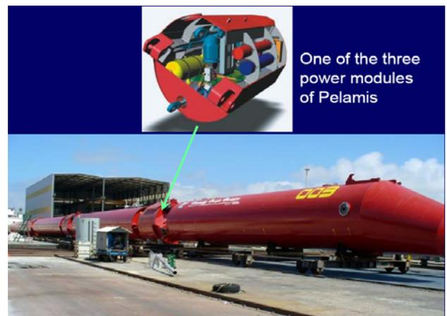
Fig 4 – A 750 kW<sub>e</sub> Pelamis unit, Aguçadura, Portugal (I-Source 15)
