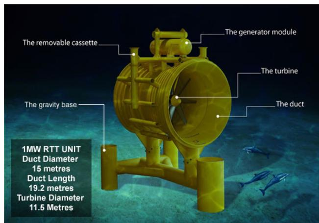
Fig 9 - Scheme of tidal stream power unit - Lunar Energy, UK (I-Source 32)
