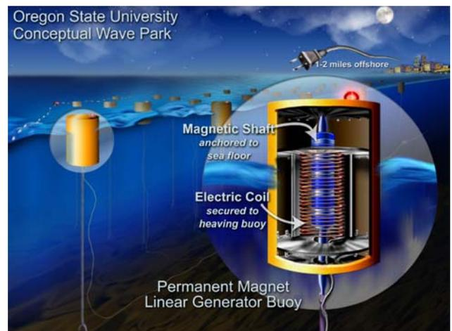
Fig 3 - AWS point absorber generator concept - Oregon State University (I-Source 9)
