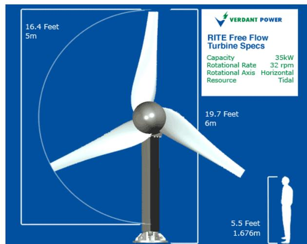
Fig 6 - Verdant Power power unit scheme (I-Source 26)
