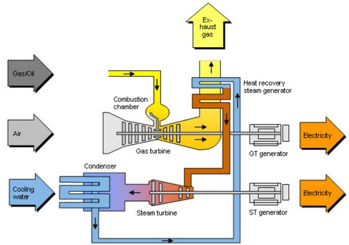
Fig. 1 - Gas-fired CCGT plant (Siemens, 2008)
